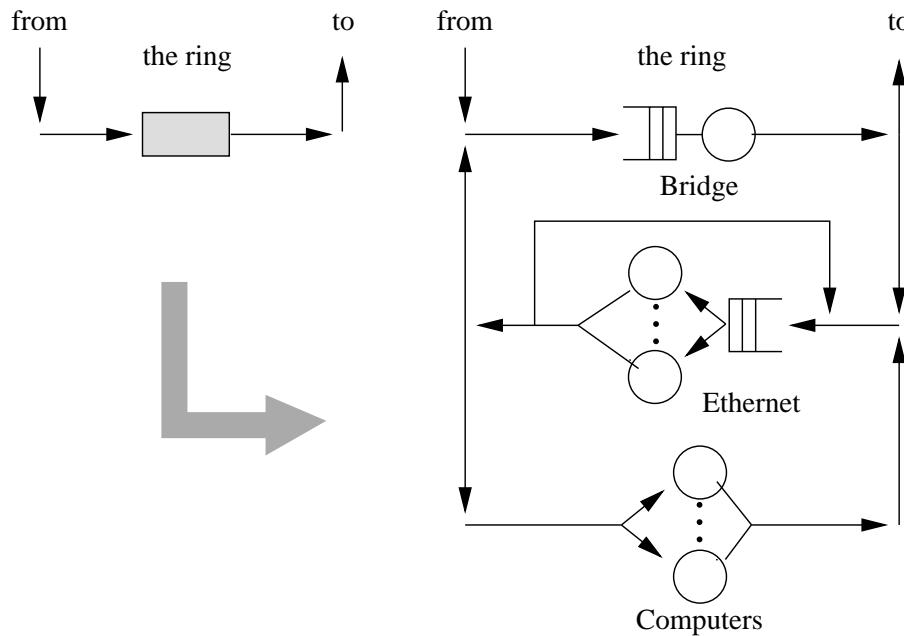
◆ Model of a section of the LAN with servers:
