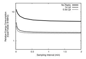
Fig. 3. Relative energy consumption of Opal vs. TelosB running a low-duty-cycle, periodic sensing application at different sampling intervals with low-power listening
