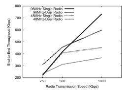
**Fig. 2.** Throughput of a data streaming application for different radio and MCU speeds. The application consists of a single node transmitting back-to-back packets through a basestation node connected to a PC via a USB link, using either one (RF231) or two radios (RF212, RF231) with bitrates between 0.25 and 1 Mbps on each radio. The MCU speed on both the basestation and the streaming node varies between 48 and 96 MHz.
